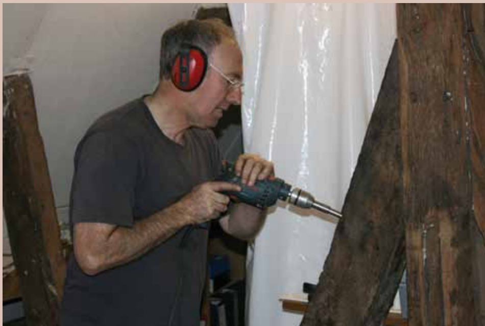
Robert Howard of the Nottingham Tree Ring Dating Laboratory taking a core from one of the Lady Row roof timbers
